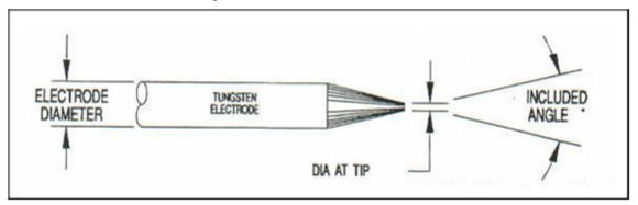
Choosing the best electrode geometry requires compromise among various attributes such as: shorter to longer electrode life, easier to more difficult arc starting, deeper to shallower weld penetration, and wider to narrower arc shape (and thus bead shape and size as well). Whichever geometry is selected, it should be used consistently as part of a successful welding procedure.
