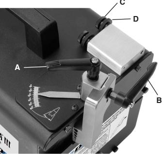
Next, put the tungsten at the diameter you plan to use through the proper sized collet hole on the universal collet and observe the height at which the tungsten will hit the wheel. For setting up your first tungsten on a wheel, make the height as close to the top of the wheel as possible by:
