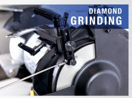
Produces a longitudinally ground taper with a 20RMS finish and a  $\pm 1/2^{\circ}$  angle tolerance.
