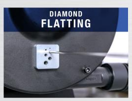
Produces a diamond ground flat surface at the tip of the electrode.
