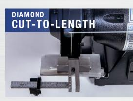
Produces smooth diamond cut electrodes on a selectable length scale.
