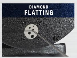
Produces a diamond ground flat surface at the tip of the electrode.
